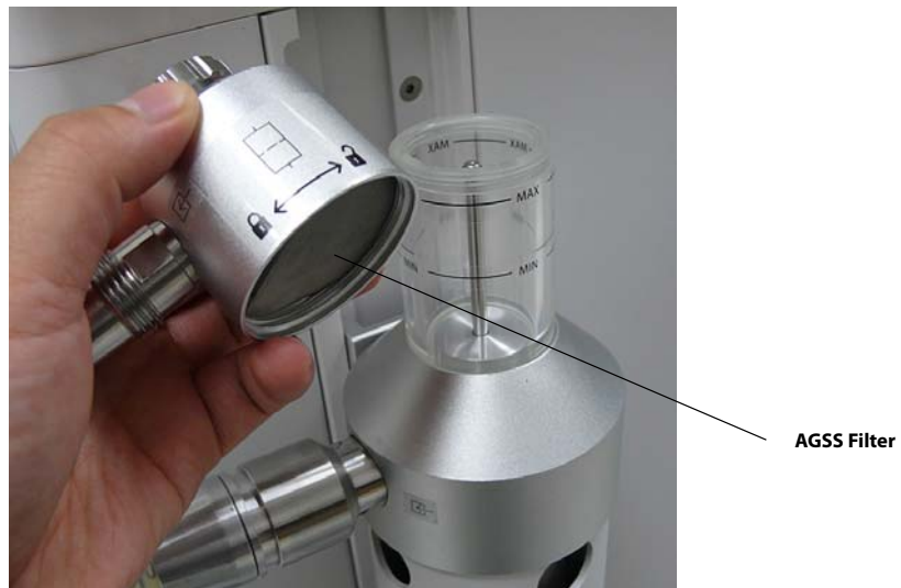
FIGURE 7-27 Removal of AGSS Top / AGSS Filter Inspection
