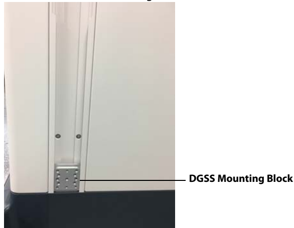
FIGURE 2-5 Install the DGSS mounting Block
