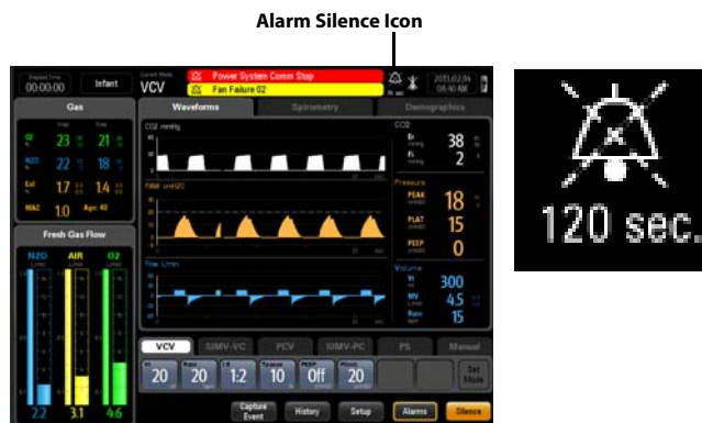
FIGURE 3-10 Alarm Silence Icon (with AG module connected)
